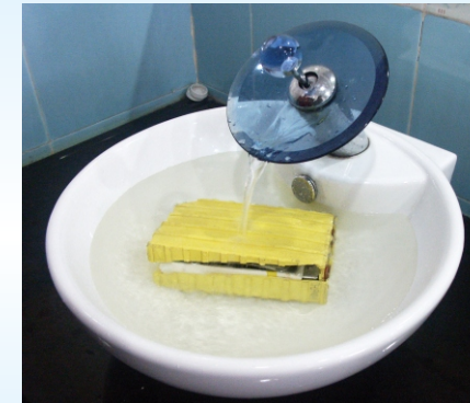
裸露的電池被水完全浸泡 Uncovered cell gets fully soaked by water
