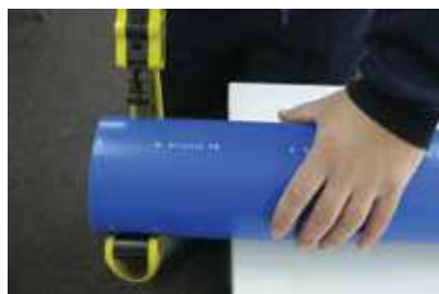
Place the cutting tool on place for cutting
