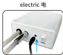
2. 电源供应线接上控制盒并开启 Plug the power cord to the control box and turn on
