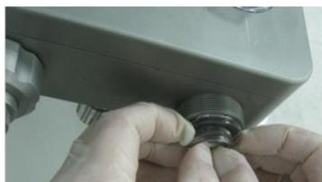
3 ) Put the respiratory connector and its locking nut together towards the inspiration flow sensor connector.
