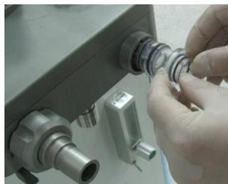
2) Flow sensor needs to be will be horizontal inserted in
