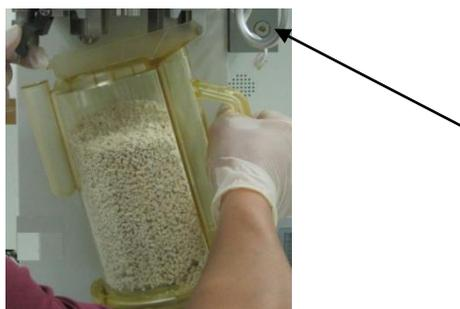
2) Press the release pin, the port Soda Lime tank are respectively aligned to push upward the absorption tank, installation in place, will release the pin lock the absorption tank.
