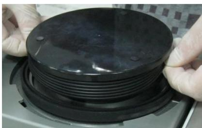
3) put the bellows cover card edge alignment card slot of loop, cover the bellows , to ensure that the bellows cover uniform pressure on the seal.
