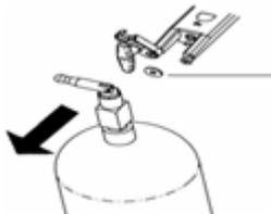
2) in front of the new bottle exit , do not place any article may due to the high pressure gas release and easily damaged.
