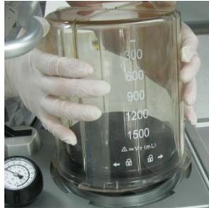
4) Both hands gripping the external side of the cover, along the clockwise, make sure that the side with scale mark towards the operator.
