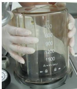
3) Remove the folding bag from the base seat of the bellows.
