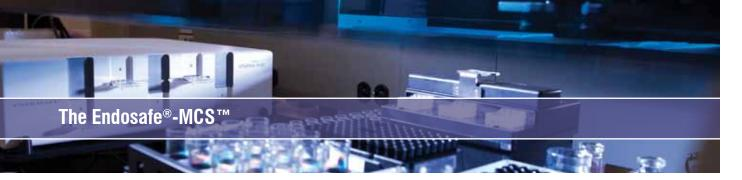
The Endosafe®-MCS<sup>™</sup> enables you to test up to five samples simultaneously. The MCS<sup>™</sup> uses our FDA-licensed disposable LAL cartridges to provide endotoxin determinations in 15 minutes. The system allows random access of samples so you can run them as needed, rather than wait for a full batch. This greatly reduces downtime and improves overall efficiency. The MCS<sup>™</sup> also links to the EndoScan-V<sup>™</sup> and Microtrend software for sample tracking and trending.
