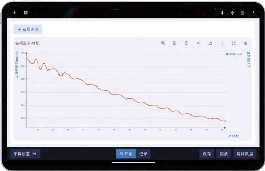
The change of ammonium ion concentration in the process of adding alkalisolution to ammonium salt
