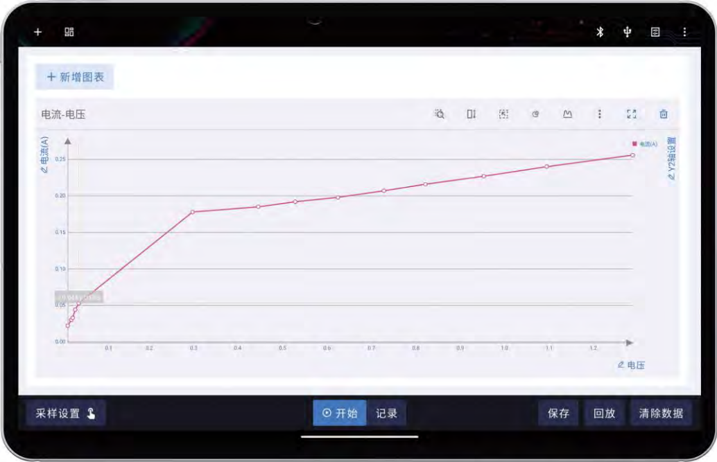
Voltammetry characteristic curve of triode
