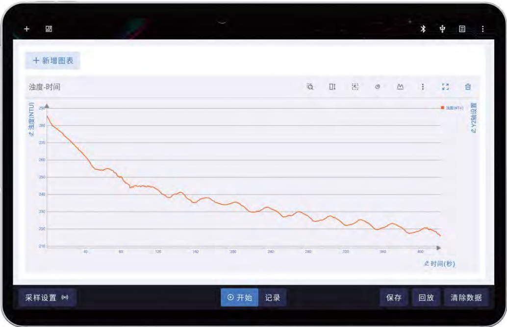
Investigate the change of turbidity in the process of static suspension
