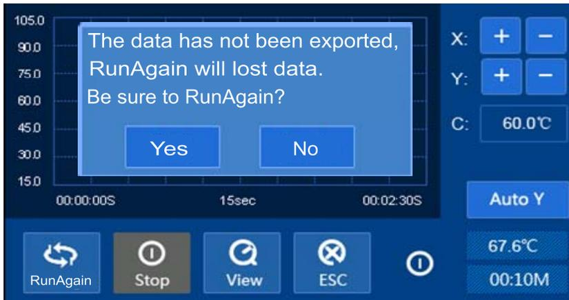
Press “Yes” to run again the current program, the data saved in the instrument will be deleted permanently (replaced by new running data). Press “No” to quit running, instrument will remind user to insert U disk and export data.
