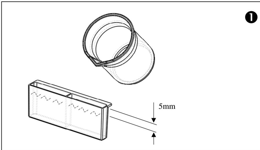
Put the tank (with purified water) at two sides of heating plate.
