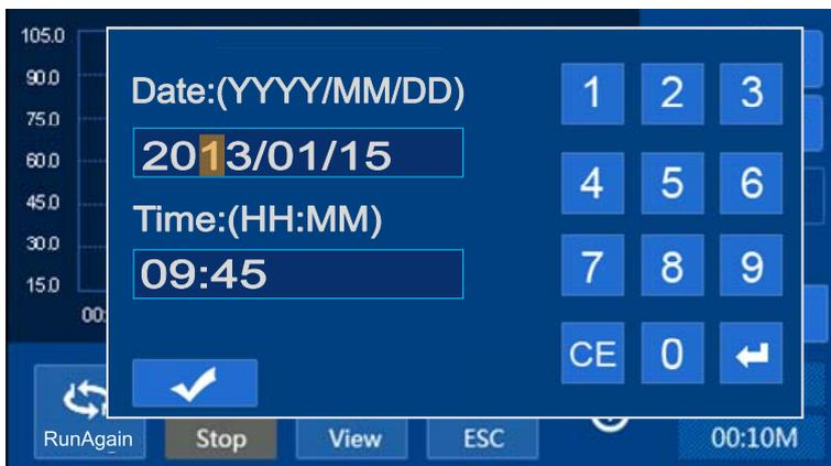
5.2 If no U disk inserted into the USB port before running, press “
