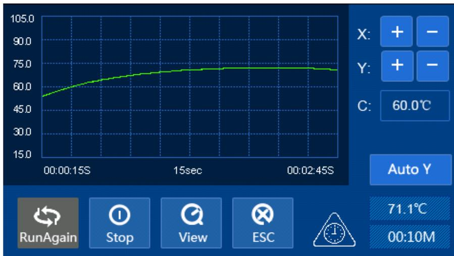
Press “Run”, the instrument will heat up to the setting temperature and the waiting notice window showed on screen, after the temperature reaches, click Start to continue.
