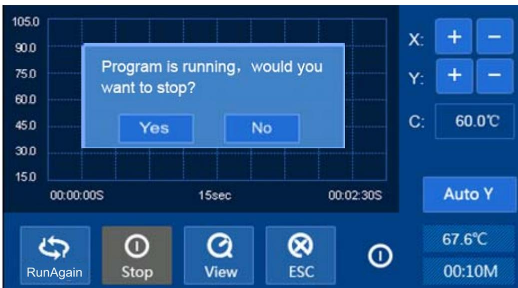
After stopping program, "RunAgain" key can be pressed to run program again. Press "ESC" to exit the program running interface and returns to main menu.
