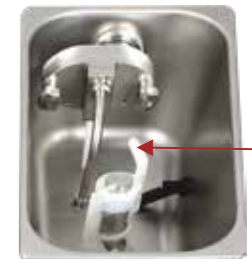
Pump in the hopper
