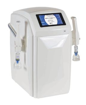
Attached G1 ultrapure water dispenser – delivers consistently ion free and low TOC ultrapure Grade 1 water.
