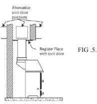
Purpose-made soot doors and inspection lengths are available from your local fireplace specialist or installer. Ensure that the whole length of the flue can be reached from the soot door.
