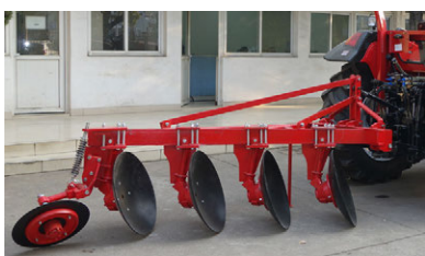
Heavy-duty one-way disc plough
