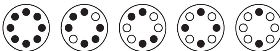
Symmetrically balanced placement of 12-, 8-, 6-, 4- and 2-tube angles (Figure 1)
