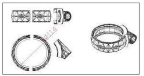
The carrier clamps can be made based on fiber polyemide (nylon 66) made by injection method or by connecting the platform directly to the carrier system. All fasteners must be disassembled and detachable.
