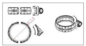
The carrier clamps can be made based on fiber polyemide (nylon 66) made by injection method or by connecting the platform directly to the carrier system. All fasteners must be disassembled and detachable.
