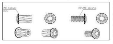
Such bolts, washers and nuts used in the system must be dachromate coated. And certainly there should be no sharp corner protrusions more than max 3mm. All nuts should be fiberglass. In this way, the problem of loosening and falling of the nuts due to vibration will be eliminated.
