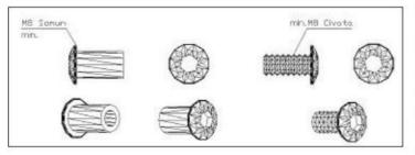
Such bolts, washers and nuts used in the system must be dachromate coated. And certainly there should be no sharp corner protrusions more than max 3mm. All nuts should be fiberglass. In this way, the problem of loosening and falling of the nuts due to vibration will be eliminated.
