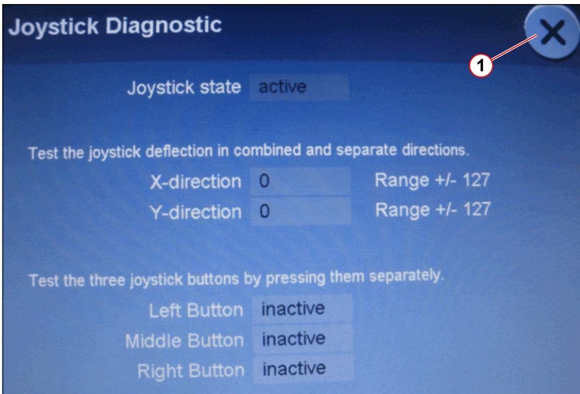
7. Once all functions have been tested, end the test at the ECC (→ 1/ Fig. 16 Page 32).
