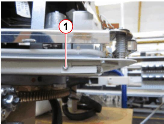
(1) Tighten the screw (ISO4762, M3x6)
