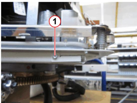
(1) Loosen the screw (ISO4762, M3x6)
