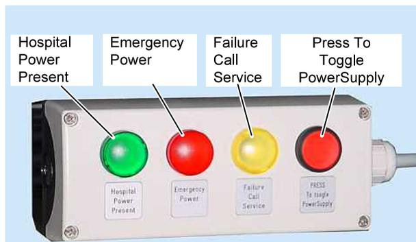
The model used for the emergency power supply mode, e.g. Powerware 9305 /9330 UL with Automatic Transfer Switch (ATS), combines a pure UPS mode for control of the Angio system with an uninterruptible switch-over of the generator from the line power to the UPS voltage, i.e. this is an emergency power supply for the complete system, incl. fluoroscopy for a period of approx. 10 min. during a primary line power failure.
