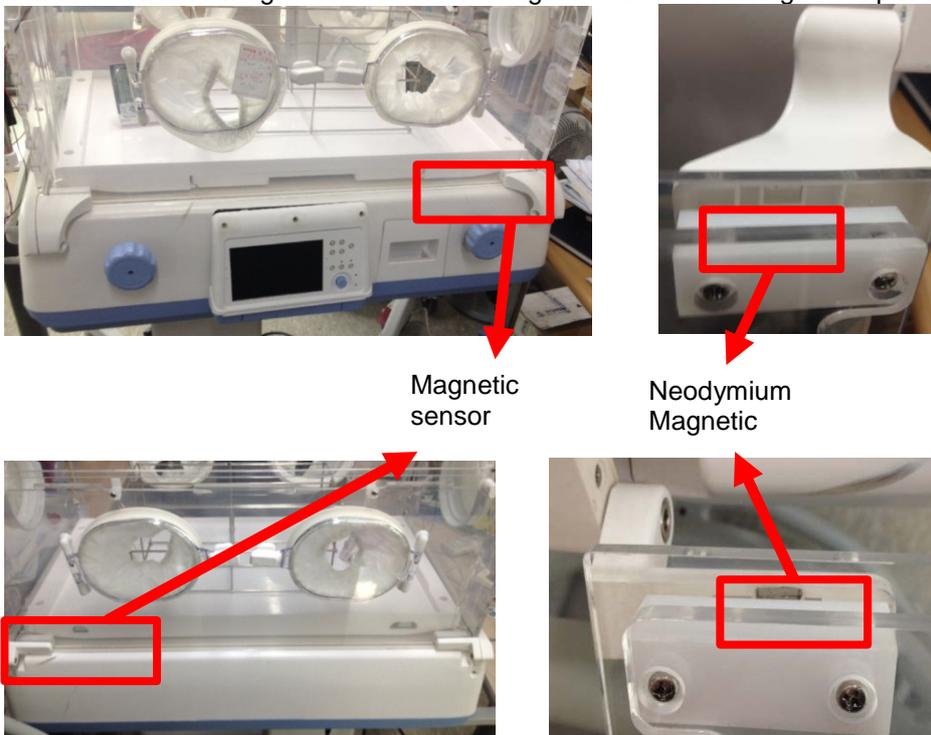
When there is a problem with the hood door sensor, check the position of magnet referring to the above picture.
