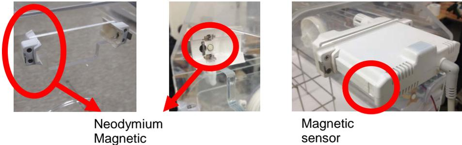
When the message “Sensor Mod Not in Position” displayed, check the magnet is in the correct position.
