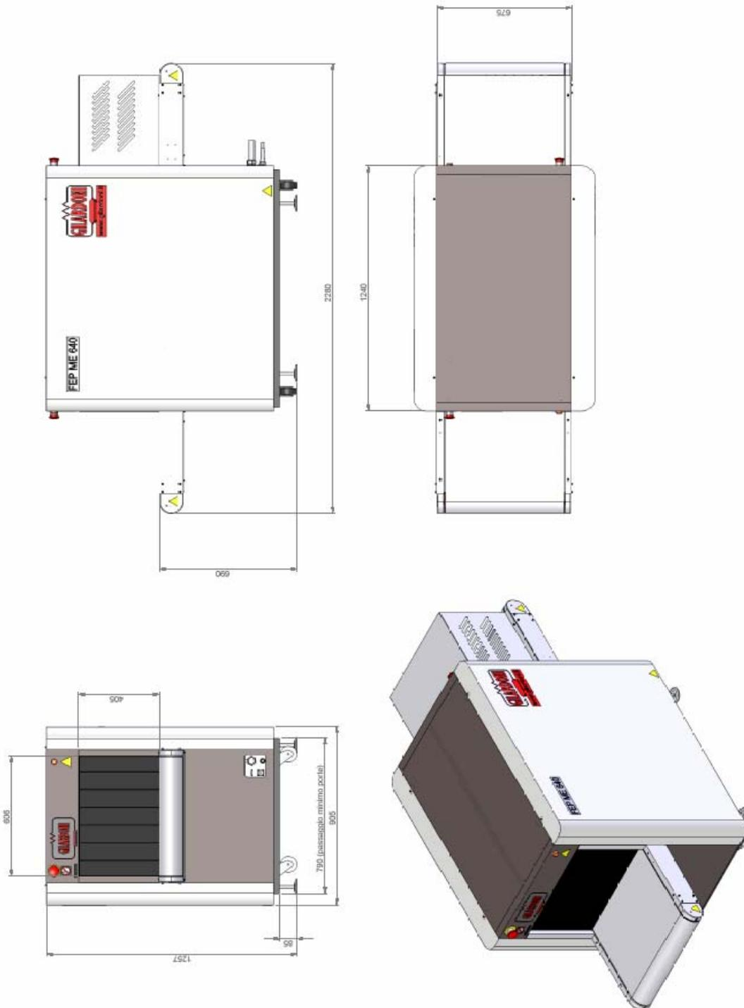
Figure 23 – Appearance and dimensions of FEP ME 640/640 LP
