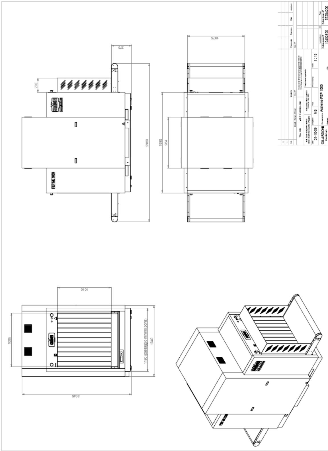
Figure 30 – Appearance and dimensions of FEP ME 1000
