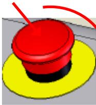
Activating one or more of the emergency buttons immediately cuts the power supply to the moving roll or x-ray emitting system.
