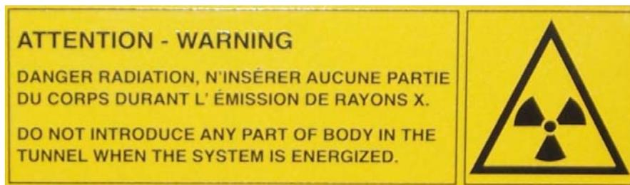
3. Label signalling the danger of putting any part of the body inside the tunnel. There are 2 labels of this kind, located over the entrance and exit of the inspection tunnel.
