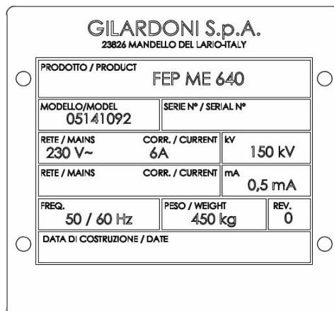
Figure 14 – Identification plate of FEP ME 640 system
