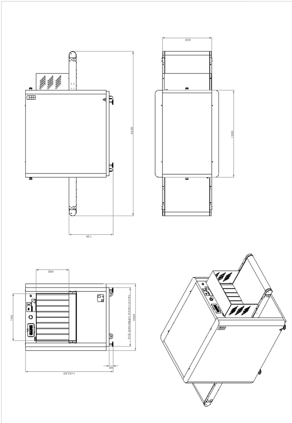
Figure 26 – Appearance and dimensions of FEP ME 755
