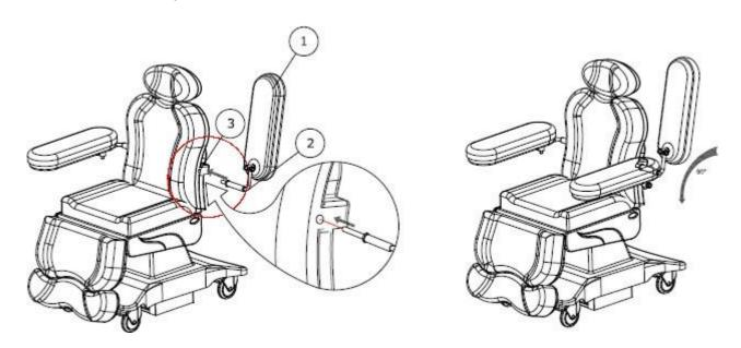
**To Install Waist Support**; remove the waist support(1) inside of the box. You can use the waist support when the chair is on any position by replacing with hand.
