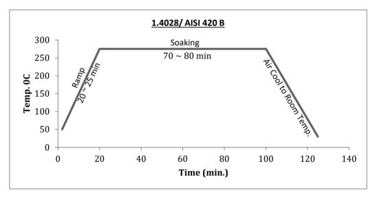
From above experiments, it is concluded from the above graphs that the time at the set temperature is most important factor. First optimal tempering furnace settings were established: ramp time 20 - 25 minutes, set temperature  $275^{\circ}$ C, and time at set temperature varies from material to material and hardness requirements from 45 - 80 minutes.
