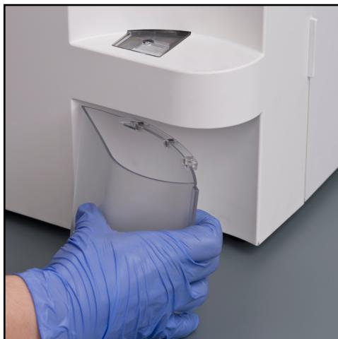
**Fig. 38:** Do not leave any used cuvettes in the waste drawer at the end of the day. Use the overhanging flap of the waste drawer to grip it and take it off the analyzer.
