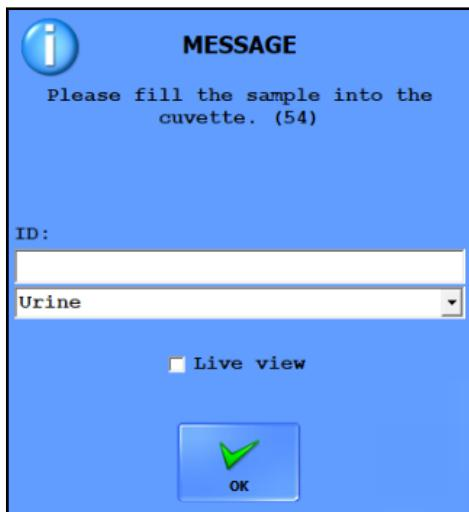
**Fig. 35:** When the cuvette is in the pipetting position, a message prompt appears. Scan the barcode or type in ID. Click OK and push the start button again to start cuvette processing.
