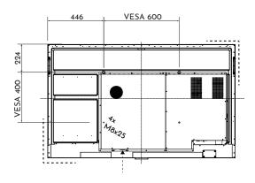
**5mm safety around display** for static elements to deal minor changes in dimensions and avoid any mechanical stress
