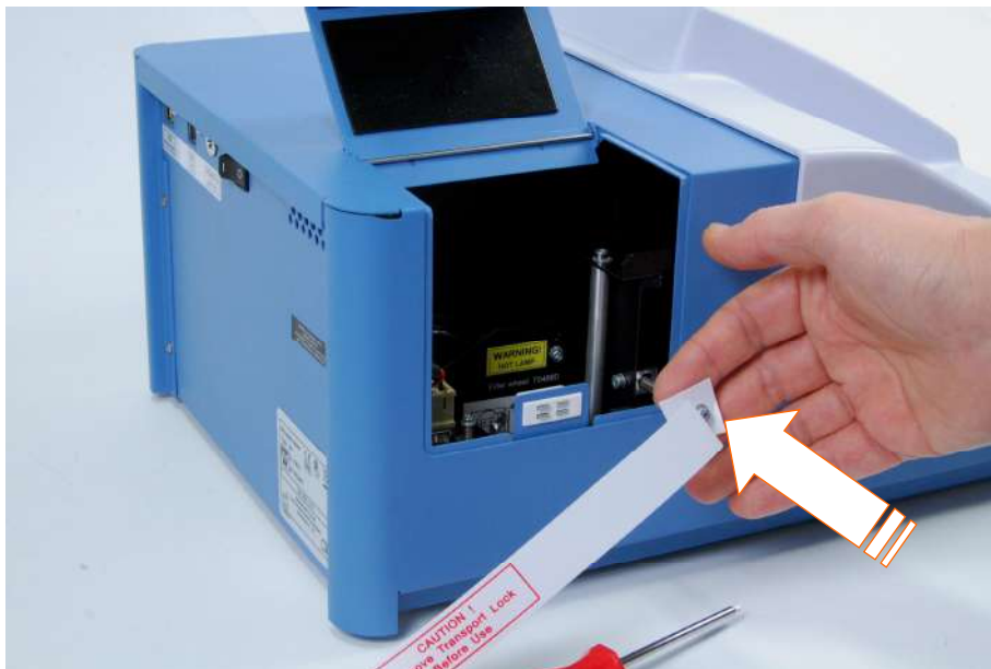
Figure 27. Refitting the transport lock bar into the measurement head
