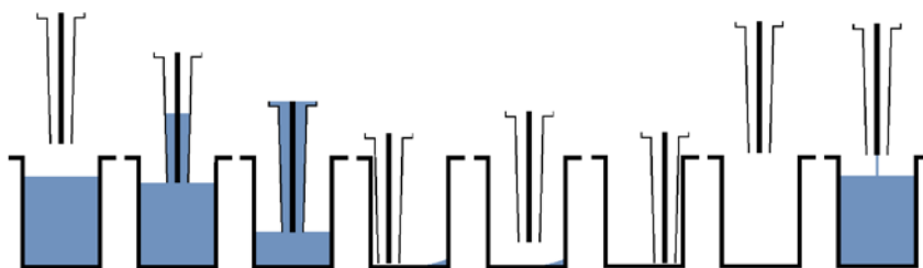
Figure 4. Principle of Wash step (Sweep2)
