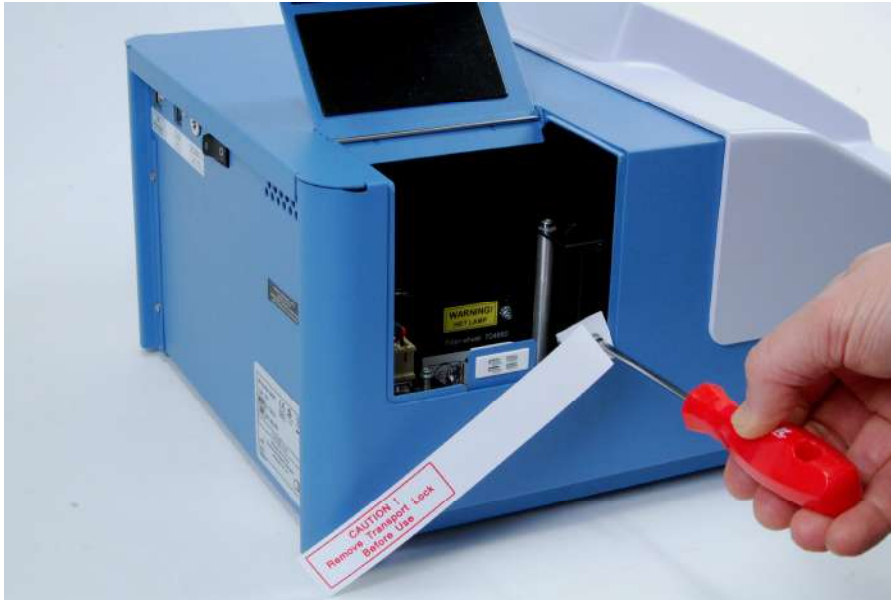
Figure 4. Unfastening the transport lock
