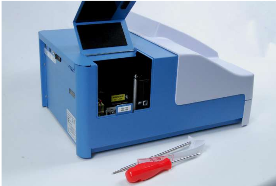
Figure 6. Transport lock bar and tag removed
