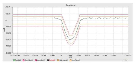
Pulse Duration: 11 ms+ Shock Type: Half Sine Mag: 300.00 m/s2 Current level: 100 % Demand peak: 300.000 m/s2 Control per Block Size: 1024 Frame Time: 0.1707 s dT: 0.000166667 s d Current Pulses: 3 Output pulses: 12 Remain pulses: 0+ Control peak: 301.797 m/s2+
