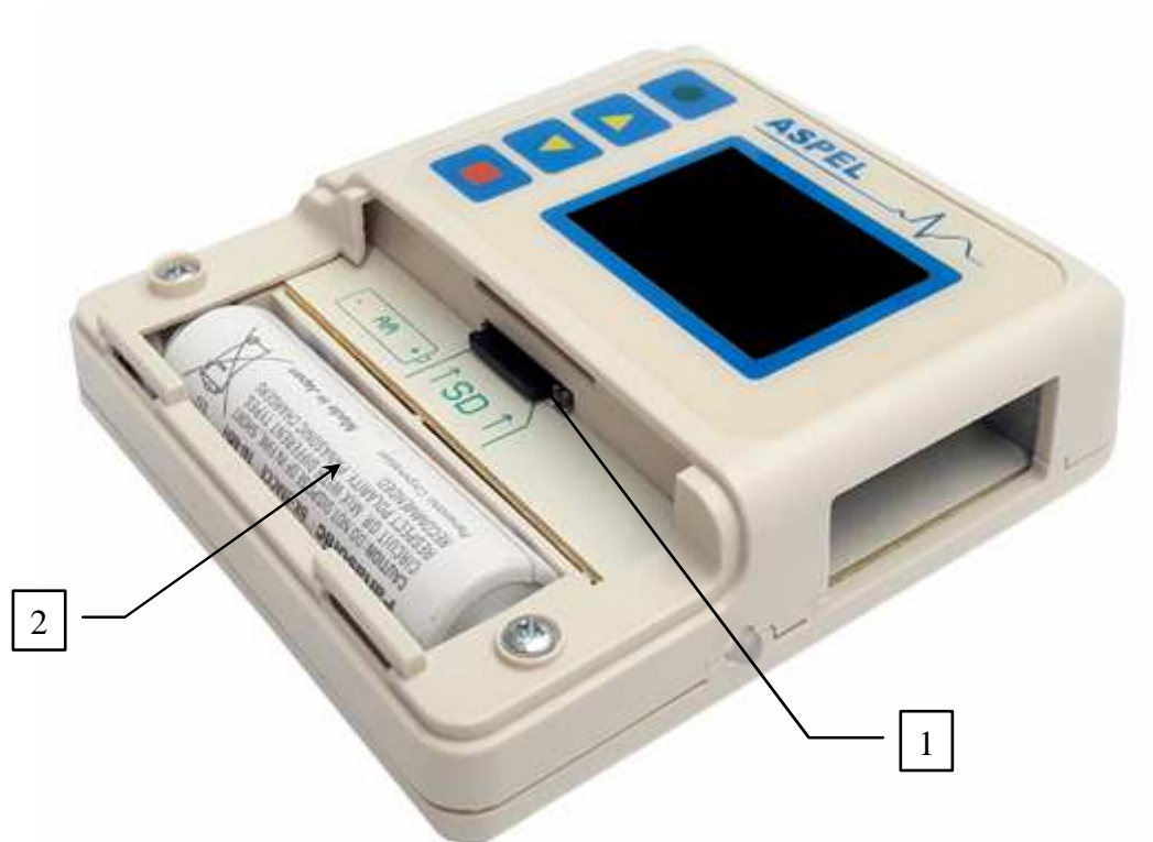
Fig. 3. AsPEKT 712 v.3xx recorder – card slot and battery socket view
