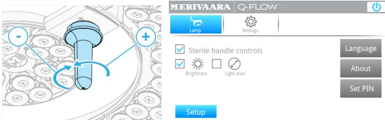
Picture 4. Simplified sterile focus handle in F-model
