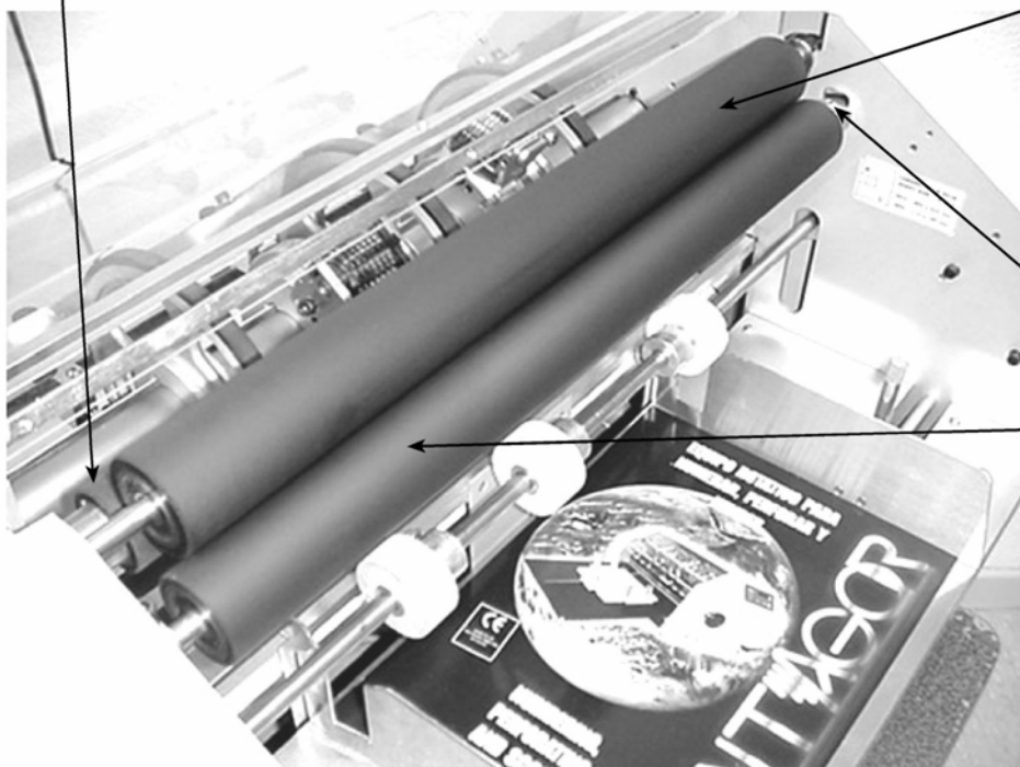
BATERIA DE RODILLOS PARA TINTA OFFSET-Modelo B INKING SYSTEM BY ROLLERS FOR NORMAL OFFSET INK-Model B
