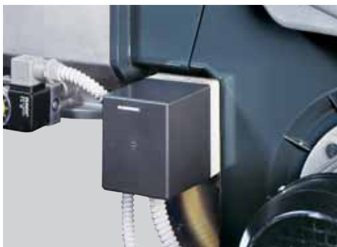
Example of the servomotor for gas setting.
