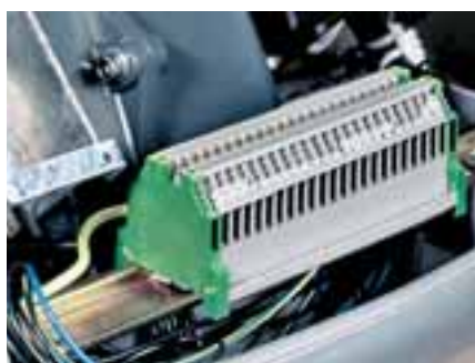
Example of the terminal board for electrical connections for the RS 70-100-130-190-250/M models.
