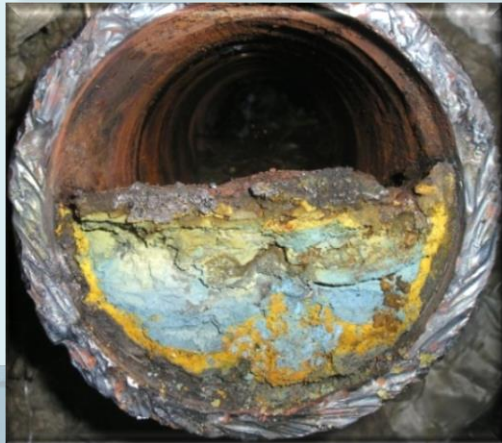
Pipes with deposits on internal walls
