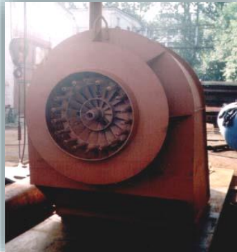
Oil-gas burner GMU-m with tubular gas distribution
