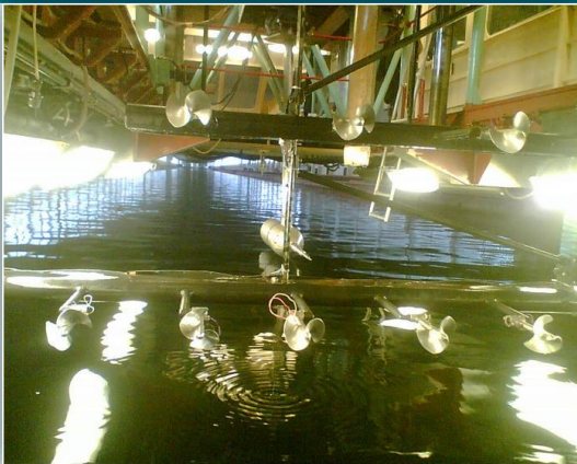
Calibration of hydrometric propellers in the pool
