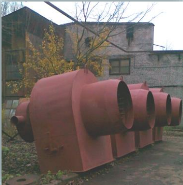
Oil-gas burner GMU-m with tubular gas distribution
