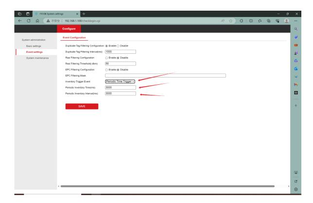
Figure 3-10 Configure device inventory trigger events
