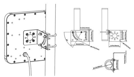
Figure 2-1 Mounting bracket
