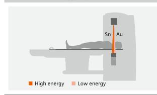
TwinBeam Dual Energy is an innovative, high-end approach that allows simultaneous acquisition of high and low kV spectra in a single spiral scan mode – with no dose penalty.
