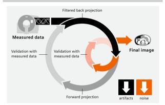
Equipped with SAFIRE, a model-based iterative reconstruction, SOMATOM go. scanners achieve up to 60% dose reduction while maintaining image quality and detail visualization combined with fast image reconstruction<sup>1</sup>. By this, equivalent results can be achieved at less dose, filling up the heat storage of the system more slowly and therefore, additionally, increasing the heat storage capacity.
