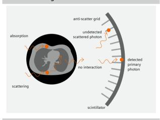
The 3D anti-scatter grid on the SOMATOM go. platform consists of thin grid walls placed between both columns and rows of the detector, all focused towards the focal spot for optimized scatter removal efficiency. The scatter signal and, consequently, the SPR decreases with the 3D anti-scatter grid by a factor of 2–3 compared to standard anti-scatter collimation with grid walls placed only between the columns. A lower SPR leads to improved CNR at a lower radiation dose.
