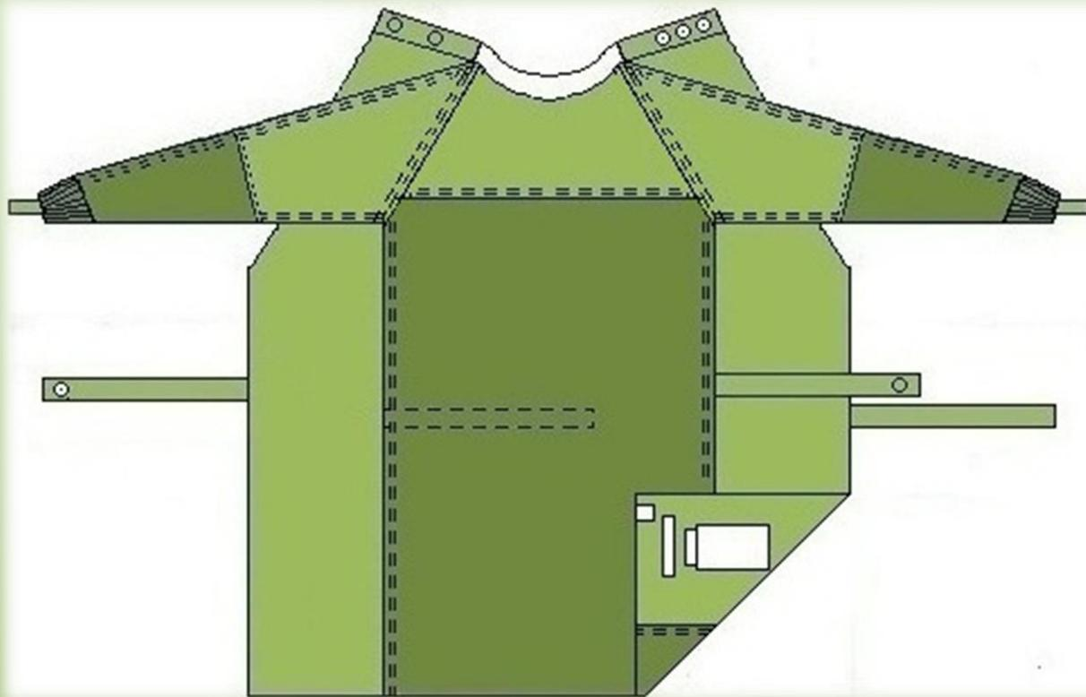
Where the critical area of the product (front and forearm) are made of tri-laminate fabric
