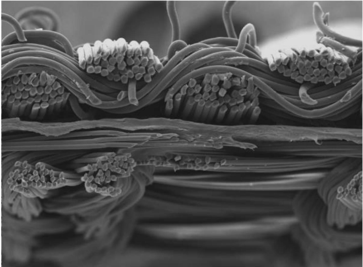
The structure of the expanded PTFE membrane is rich in micropores whose average diameter is about 0.02  $\mu\text{m}$  not sufficient for the passage of a molecule of liquid, the main vehicle for the transport of pathogens (micro holes are smaller than about 20,000 times of the water molecule; while they are larger than about 700 times of the molecule of water vapor).
