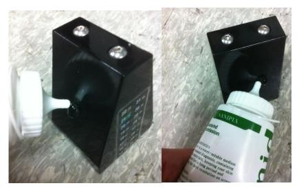
Put the phantom on the foot supporter 1 (don't use foot supporter 2 when dailytest) in the measuring position of device.
