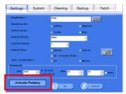
The button of Activate is used to toggle between PEDIATRY mode to BMD mode.
