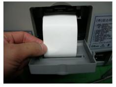
4) Paper cutting : For a sharp outline of report printing, cut off the remained paperonce by a saw tooth in the cover.
