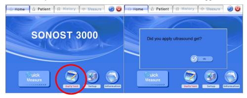
After click the daily test button, you can see the message. If you put the ultrasound transmission on the phantom, press "YES" button. Input the temperature referring to the thermo label on the surface of the device.
