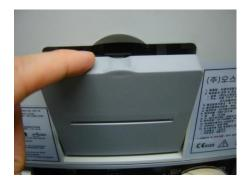
Paper inserting : Insert the paper as shown below. Outer surface of paper should face to the inside of the device. Paper isscrolled inautomatically.
