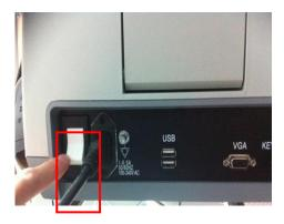
Turning off the main switch of the system
