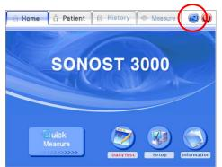
Press the screen rotation button on the top right side of the screen
