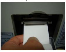
3) Cover shutting : Put the paper to the gap in the cover, then shut the coverup.
