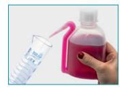
Dispensing tip provides extra fine stream. The tip of the delivery tube can be cut in order to increase the liquid flow rate.
