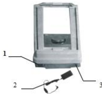
1. Data Interface 2. Transformer 3. Electrical Outlet
