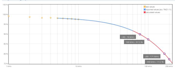
LxB50 results according to LM-80 and TM-21-11 procedures and norms.
