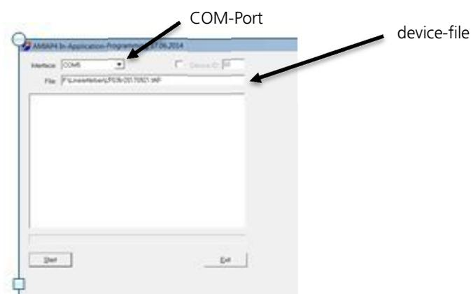
In the upper left corner, the COM-connection is shown. Click into the small window below to choose the device file for updating the linear stainer.
