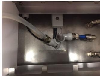
The running water cuvette can simply be clicked into the water tube at the button of the station. It can be freely selected.
