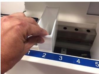
The reagent cuvette can simply be placed at the any station
