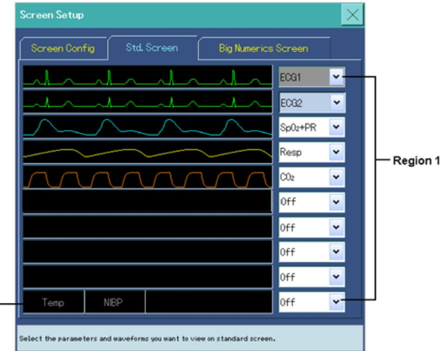
Figure 3.3 Standard Screen Layout Setup
