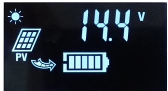
6. Floating charge voltage setting
