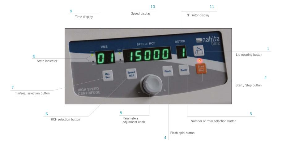
high speed multirotor centrifuge equipment parts
