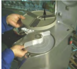
Installation of the cutting plate (4)
