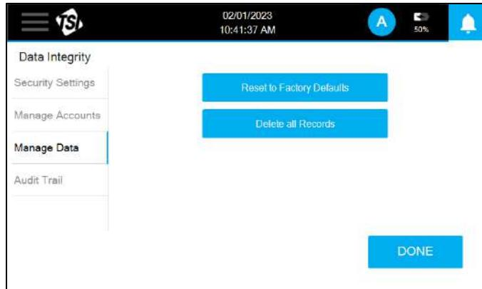
Press the **Delete all Records** button to clear all the sample records in the internal memory buffer; there is no method for selectively deleting data. Pressing the **Reset to Factory Defaults** button resets all instrument configurations to the original defaults; all records must be deleted prior to performing a factory reset. A warning box appears to confirm prior to executing the reset.
