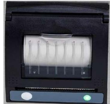
When installing a new roll of paper, the tag end should be from the bottom of the roll and pulled through the printer door.
