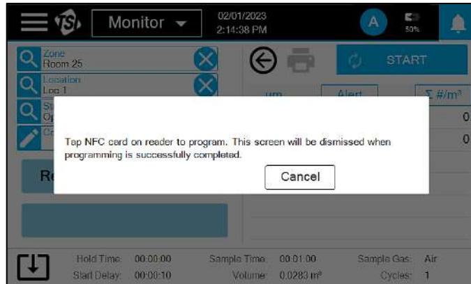
Hold an NFC card near the NFC Reader/Writer. The prompt will be dismissed and a beep will sound to indicate the card has been programmed.
