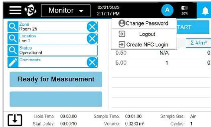
A prompt will appear. Hold an NFC card near the NFC Reader/Writer. The prompt will be dismissed and a beep will sound to indicate the card has been programmed.
