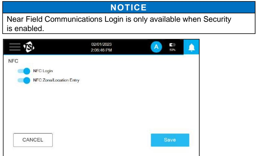
With NFC Zone/Location Entry turned on, an NFC card can be programmed by going the Sample screen in either Monitor or Classify mode. Select a Zone and Location and tap the
