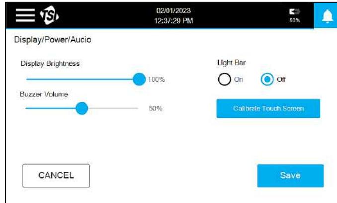
Use the sliders to adjust the Display Brightness and Buzzer Volume. The Light Bar can be turned On or Off. If the touchscreen responsiveness has become poor, it can be calibrated to try to improve performance. Press the **Calibrate Touch Screen** button and follow the prompts.
