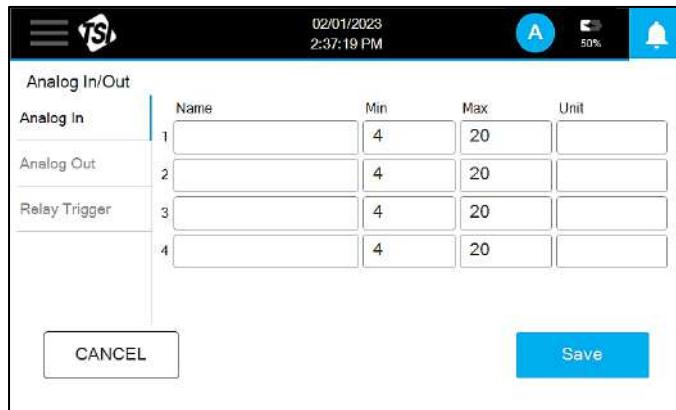
The screenshot shows the 'Analog In/Out' configuration screen. The 'Analog In' tab is selected. There are four rows for analog inputs, each with fields for 'Name', 'Min', 'Max', and 'Unit'. The 'Name' column contains empty text boxes. The 'Min' and 'Max' columns both have the value '4'. The 'Unit' column is empty. At the bottom are 'CANCEL' and 'Save' buttons.
