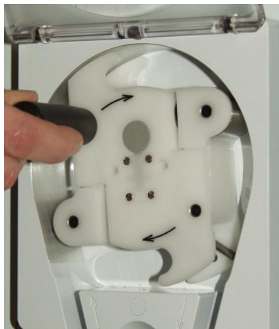
Fig. 13-3 Use of crank (alternative 1)
