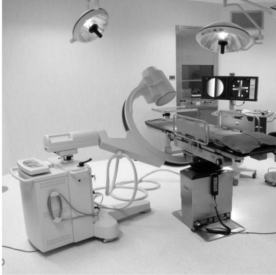
This equipment is a highly optimized mobile System for surgical fluoroscopy. The optimization is the pursuit of the best compromise within the peculiar features of such an instrument : dimensions, weight, balancing, ease of manoeuvre, X-ray features, image quality, safety.
