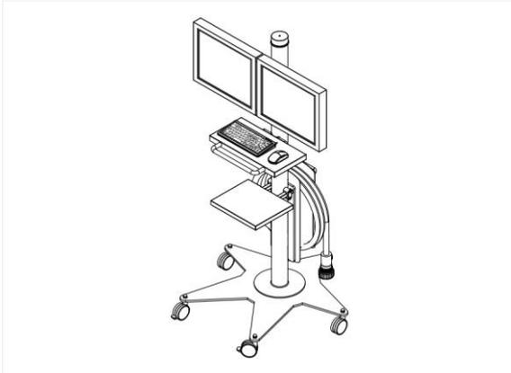
Display station with one/double 19" LCD monitor for video systems 0,5K<sup>2</sup>
