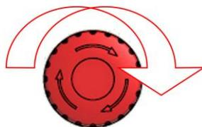
The mushroom emergency pushbutton on the display station stops the power supply to the whole equipment.
