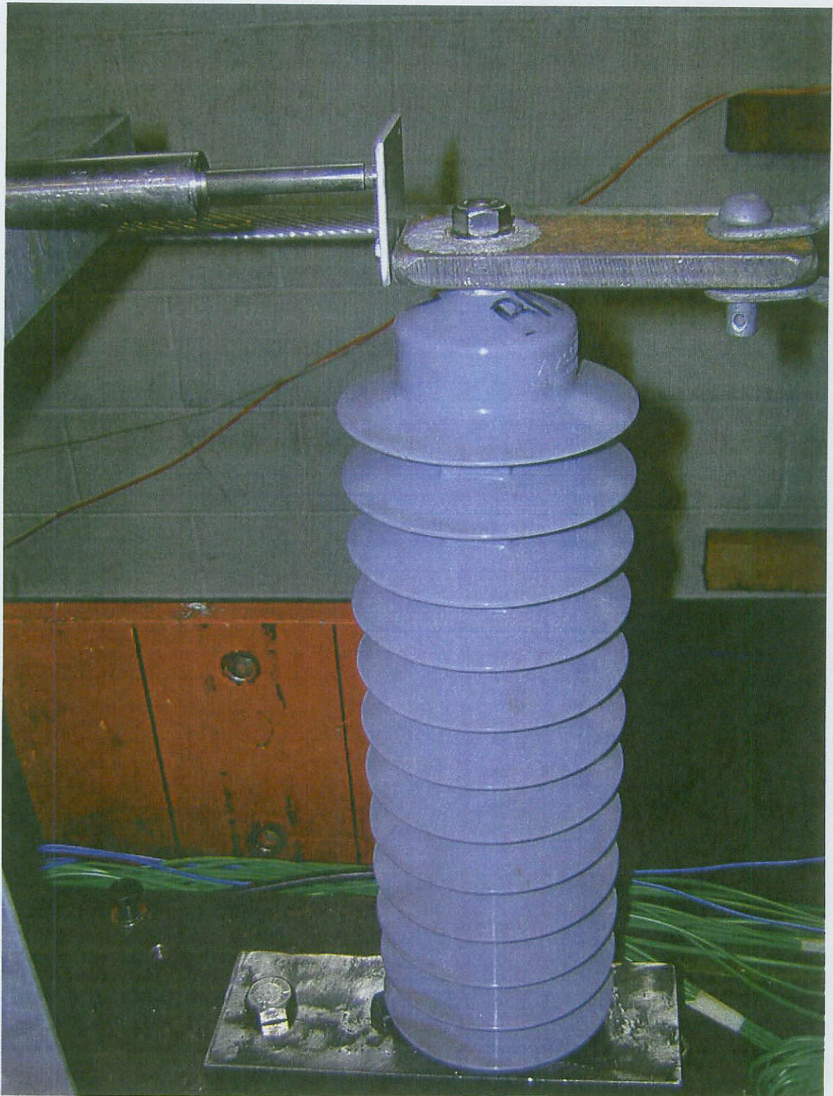
Photo no. 2 Test setting for bending application
