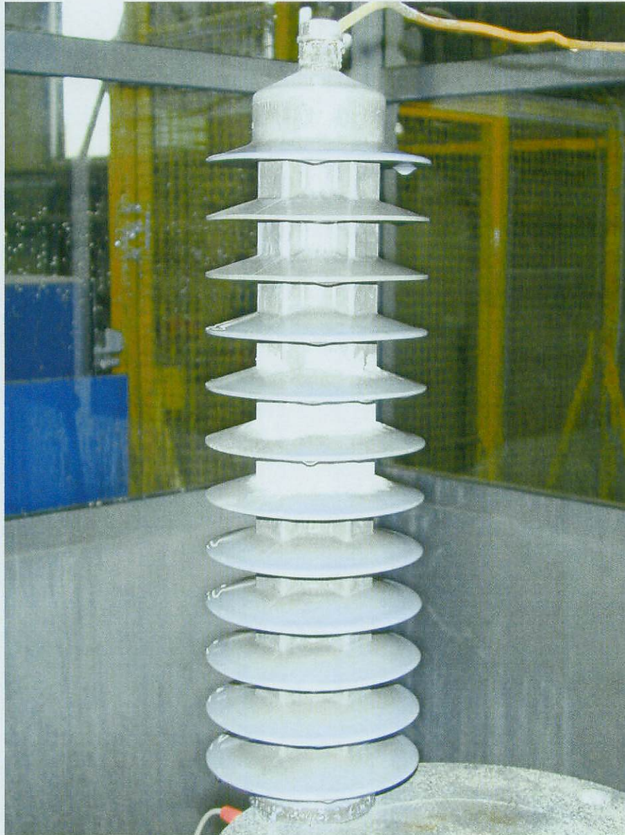
Overall view of the test sample after the weather ageing test
