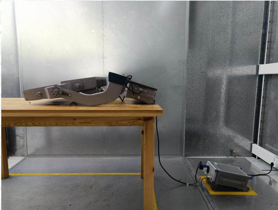
Figure 3: Conducted Emission Test Setup
