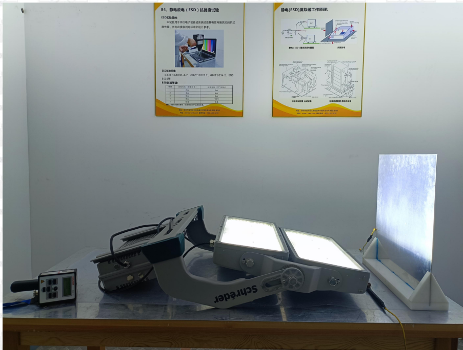
Figure 5: Electrostatic Discharge Test Setup
