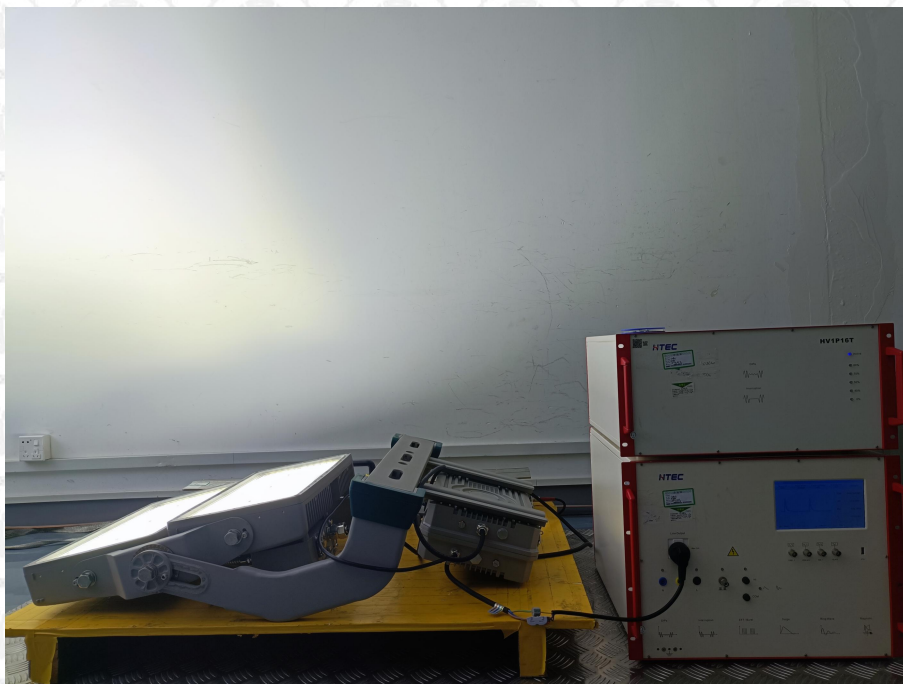
Figure 6: SURGE、DIP&EFT Test Setup
