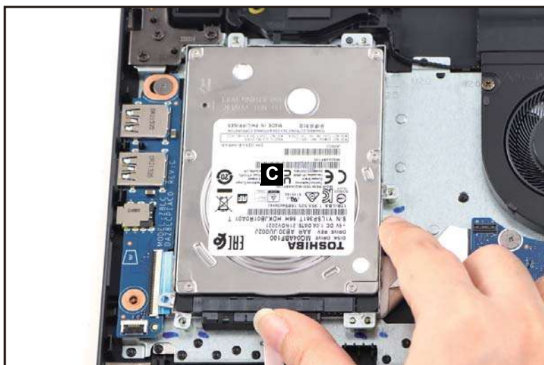
Figure 3-35. HDD Module Removal
