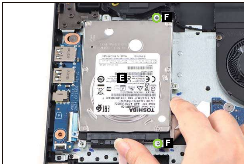
Figure 3-101. Replacing the HDD Module
