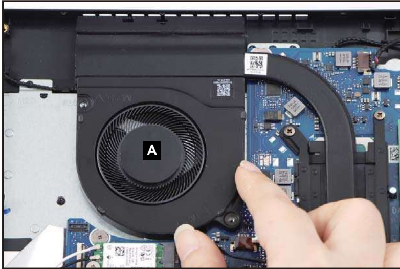
Figure 3-107. Replacing the Fan
