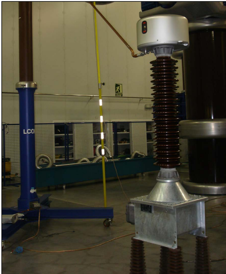
Picture 1.2 – Voltage transformer UTD-123.
