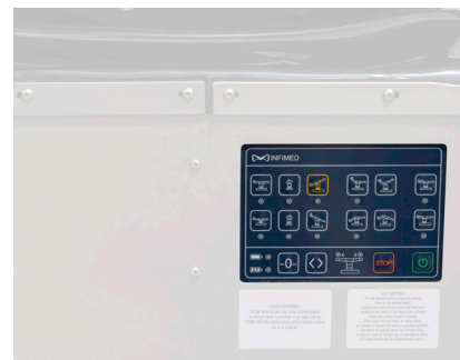
Sensor side control panel
