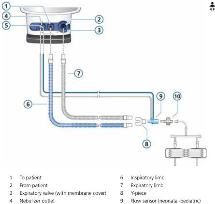
Figure 5-4 Dual-limb breathing circuit with HMEF/HME (neonatal)
