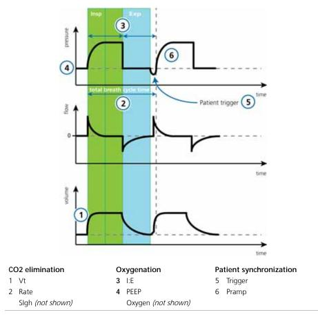
Figure B-4 APVcmv / (S)CMV+ mode: Breathing pattern and controls
