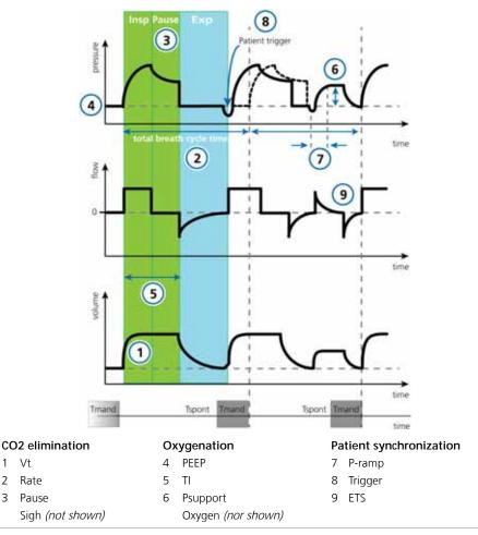
Figure B-5 SIMV mode: Breathing pattern and controls
