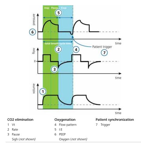
Figure B-3 (S)CMV mode: Breathing pattern and controls
