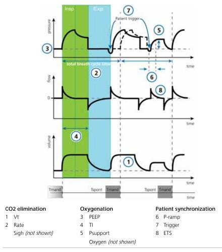
Figure B-6 APVsimv / SIMV+ mode: Breathing pattern and controls
