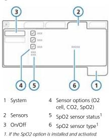
Figure 3-3 Sensors > On/Off window
