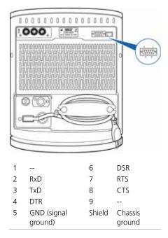
Figure H-5 RS-232 cable (PN 160366) wiring diagram
