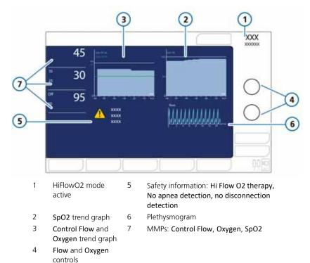
Figure 4-5 High flow oxygen therapy display
