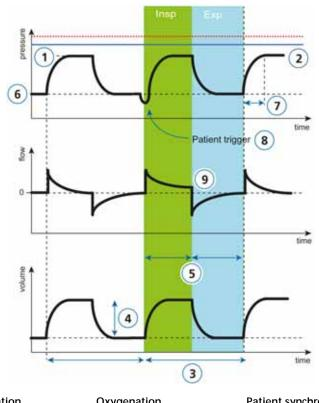
Figure B-16 **ASV mode:** Breathing pattern and controls
