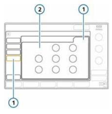
1 Vent Status 2 Parameter weaningzone settings: Oxygen, PEEP, %MinVol, Pinsp, RSB, %fspont Figure I-13 Vent Status intelligent panel
