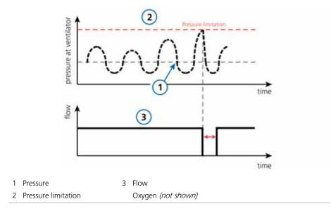
Figure B-15 High flow oxygen therapy: Breathing pattern and controls
