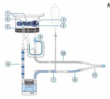
Figure 5-5 Breathing circuit with humidifier, for nCPAP-PS (neonatal)
