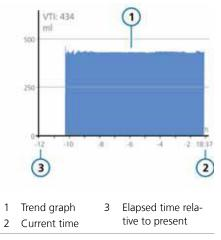
From the time you turn on the HAMILTON-C3, the ventilator continually stores up to 72 hours of monitored parameters in its memory, so you have access to any of this data, even after standby. If the HAMIL-TON-C3 is turned off, the data of the last patient is available in memory when ventilator is turned on again.
