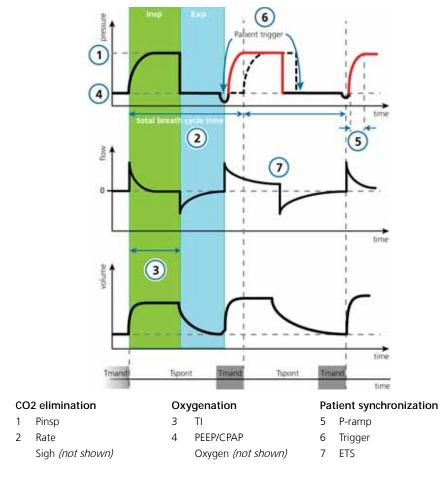
Figure B-9 PSIMV+ with PSync mode: Breathing pattern and controls
