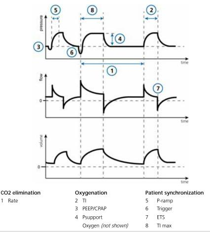
Figure B-14 nCPAP-PS mode: Breathing pattern and controls
