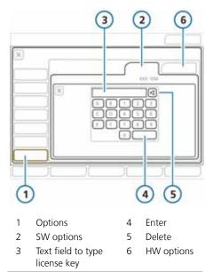
Type the activation code exactly as provided into the field and touch Enter.
