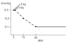
For patients with an IBW  $\ge$  30 kg, minute ventilation is calculated as 0.1 l/kg \* IBW (solid line). For patients with an IBW < 30 kg, the value is indicated by the dotted line. Minute ventilation for a 15 kg patient thus is calculated as
