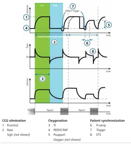
Figure B-8 **PSIMV+ mode:** Breathing pattern and controls
