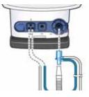
2. Connect the blue and clear tubes to the flow sensor connectors on the ventilator.
