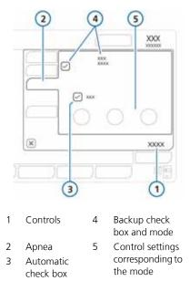
If the patient triggers two consecutive breaths, the ventilator reverts to ventilation in the original support mode and at the original settings, and it displays Apnea ventilation ended.
