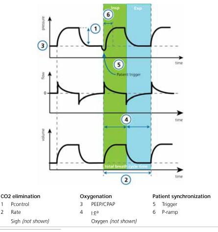
Figure B-7 **PCV+ mode:** Breathing pattern and controls
