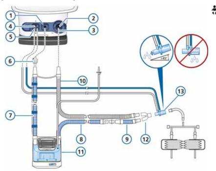
Figure 5-3 Dual-limb breathing circuit with humidifier (neonatal)
