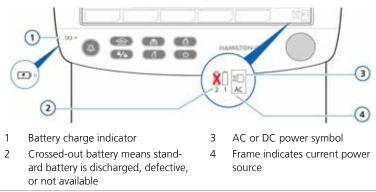
The power source symbols in the bottom right-hand corner of the screen show the available power sources. A frame around a symbol indicates the current ventilator power source. Green indicates the level of battery charge.
