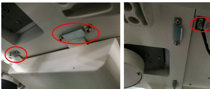
Figure 4-8 Removing Pull Keyboard Assembly
