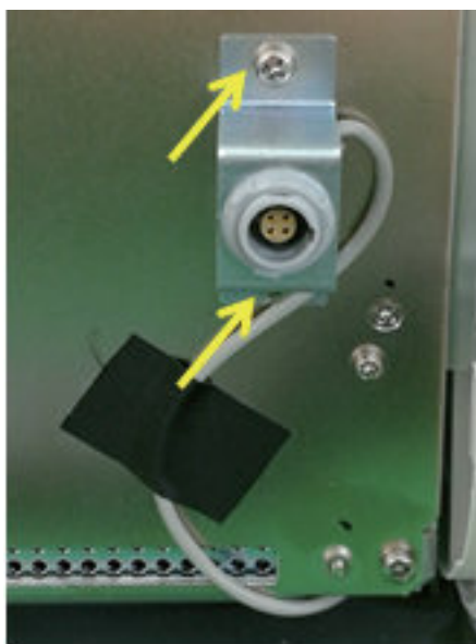
Figure 4-28 Removing Footswitch Socket
