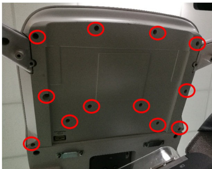
Figure 4-14 Removing Screws Fixing Keyboard Top cover
