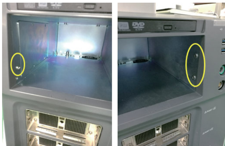
Figure 4-24 Removing Screws Fixed Printer Front Panel
