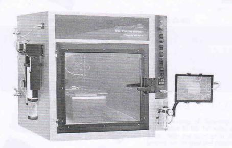
Spray pyrolysis is a process in which a thin film is deposited by spraying a solution on a heated surface, where the constituent reacts to form a chemical compound. The process is particularly useful for the deposition of oxides and has long been a production method for a long period for applying a transparent electrical conductor of Tin oxide (SnO2) or Stannic oxide to a glass. Now is popular to prepare perovskite solar cell.
